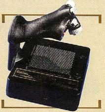
throttle can function in analog mode, or can send a series of keypresses for sims that don't have throttle support. There are two three-position switches, a four-direction radio switch, and two programmable dials. The dials can be used for any function that allows a range of settings—you might use them to change radio frequencies or control flap deployment.
