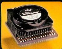
Designed to upgrade 75-, 90-, and 100MHz Pentiums (they can be used in faster machines if you're looking to add MMX), the MMX OverDrives feature a voltage regulator that adapts the 3.3v system voltage to the 2.8v required by the MMX chip; added capacitors to ensure compatibility with early, noise-sensitive motherboards; and a built-in fan and heat-sink. In addition to boosting the computer's clock
