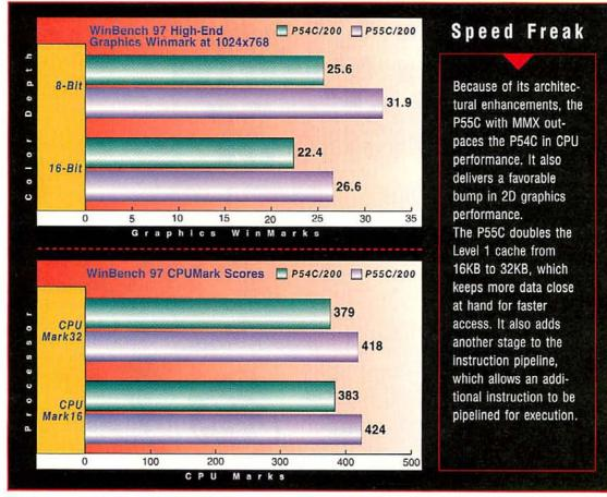
The internal (also known as Level I) cache size has been doubled to 32KB, from the previous size of 16KB. In addition, the instruction pipeline has been increased one step, which allows CPU instructions to line up, ready for execution, rather than having to be fetched from memory every time the next one is needed for use.
