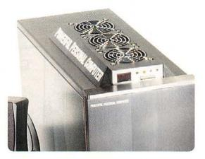
Voodoo doesn't take cooling for granted. The E-Class Glycol machine features three big fans and a digital temperature readout.
