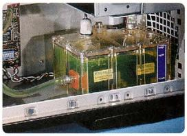
The E-Class Glycol also ships with a liquid-cooled radiator. According to Voodoo, the Glycol-filled reservoir should last as long as the machine.
